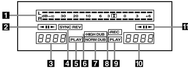
**1 Peak Level Meter** – Segments of this dual horizontal bar will illuminate to indicate the input level for recording or the output level on playback. The meter will “hold” the average constant level and flash to indicate momentary peaks.
